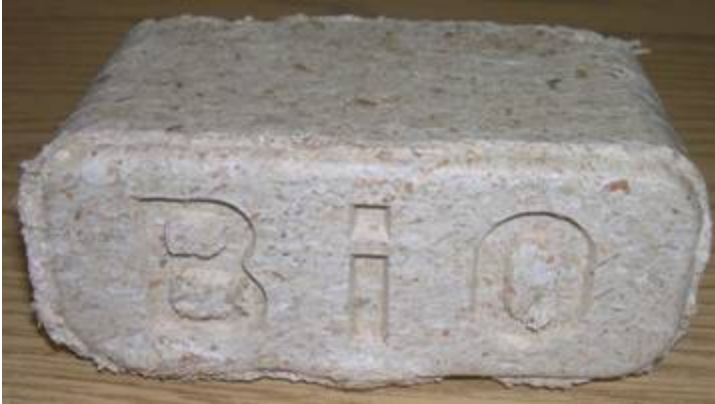
Wood chips can be used to make wood bricks (for example, BioBricks™.)
